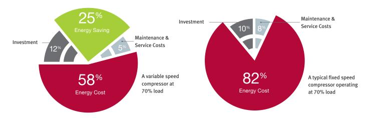
Using a variable speed compressor can easily **save 25% energy** by using just the right amount of energy required to do the job and no more.
