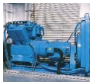
A CompAir H5336 compressor installed by Trane Company to test the integrity of its air conditioning coils.
