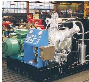
3 stage nitrogen boosting compressor being prepared for shipment to Kazakhstan as part of a nitrogen generation and compression system.
