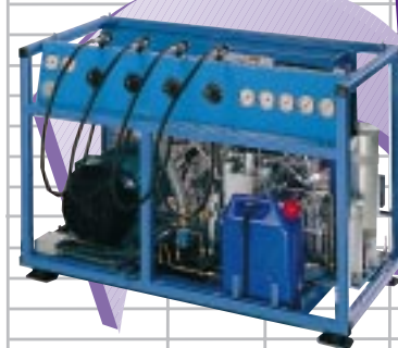
CompAir HAB30 breathing air package using a CompAir H5407 air cooled compressor. Packages for industrial and breathing air applications, compressing high quality air and gases. One in a range of seven, 3 and 4 stage models.
