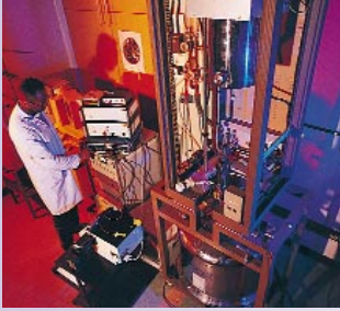
Two CompAir reciprocating compressors are playing a vital role in the recovery of helium gas for the Condensed Matter Group of the Physics Department at Birmingham University.
