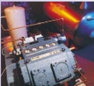
Two CompAir reciprocating compressors are playing a vital role in the recovery of helium gas for the Condensed Matter Group of the Physics Department at Birmingham University.
